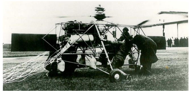
Figure 38. Test of engine cooling fan, Ref. 108.
