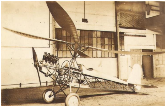
(a) Propeller and second pair of rotor blades mounted, pre-rotator clutch installed
